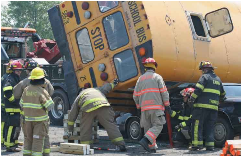
Fill all voids to ensure the heavy vehicle is stabilized and further shifting does not occur.
